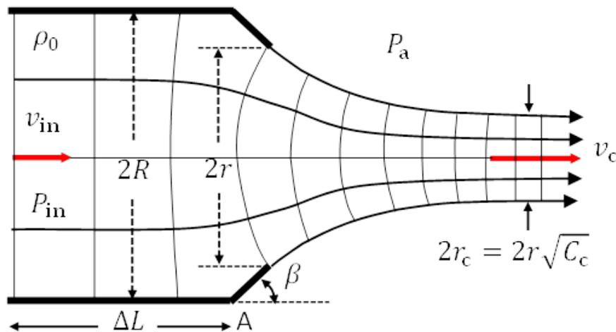
Fig. 2: Valve dimensions and contraction of jet.
