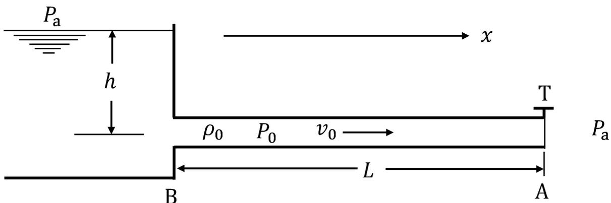
Fig. 1: Steady flow in a uniform pipe.
